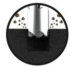
After deciding the location where the fixture will be installed, drill a hole having a minimum diameter of 9.1" (230 mm) and a minimum depth of 5.1" (130 mm).
