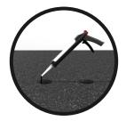
Pour ±15.4 lb. (±7 kg) of ULTRAFLOW 4000/8 grout in the hole and insert the fixture. Remove any excess grout.
