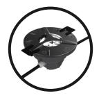
Add the installation accessory to each fixture that will be installed. The accessory will help align and keep the fixture in place during the grout drying time. This accessory will be removed at the end of the installation.
