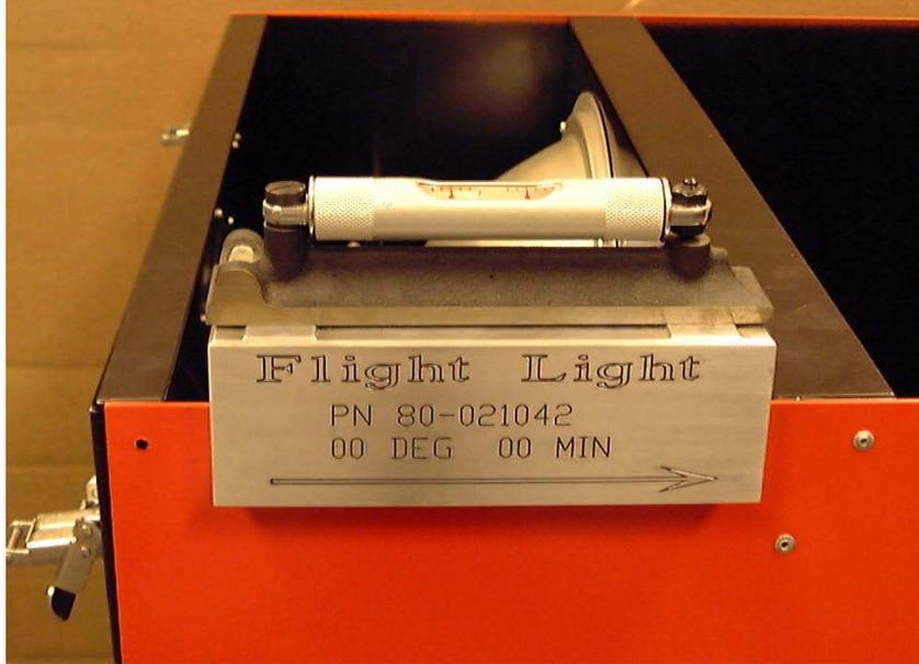
Figure 2 - Spirit level placed on Aiming Device.
